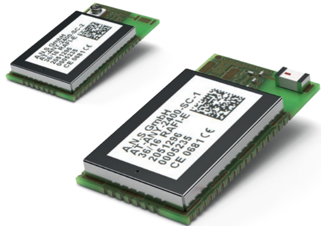
Mechanical module size 24 x 13.5 x 3 mm
