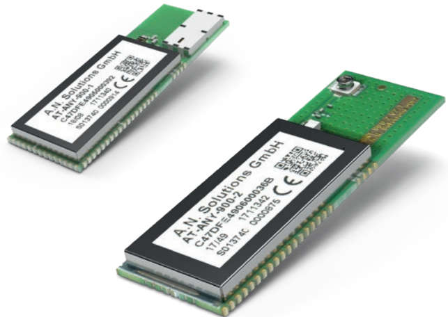
Mechanical module size 40 x 13.5 x 3 mm
