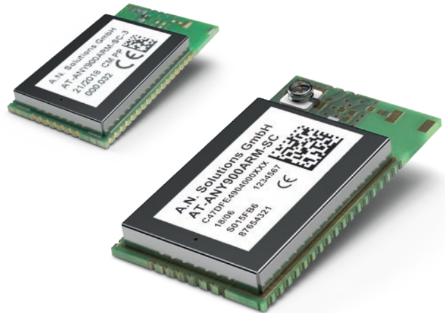
Mechanical module size 24 x 13.5 x 3 mm
